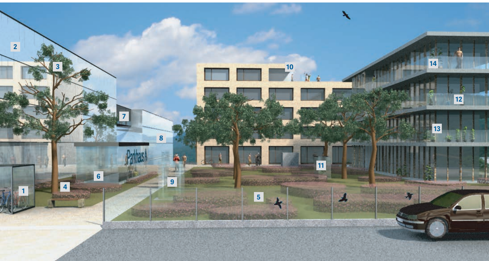
Overview of the hazards in a modern development: 1 Bicycle stand in transparent material; 2 Reflective façades (glass, metal, etc.); 3 Trees in front of reflective façades; 4 Attractive green spaces in front of reflective façades; 5 Transparent noise barriers with ineffective black silhouettes; 6 Glazed entrance to the underground parking; 7 Transparent aerial walkway; 8 Reflective façades; 9 Garden sculptures made of reflective or transparent material; 10 Transparent corners; 11 Winter garden; 12 Glass balcony walls; 13 Transparent corners; 14 Plants behind transparent surfaces.
