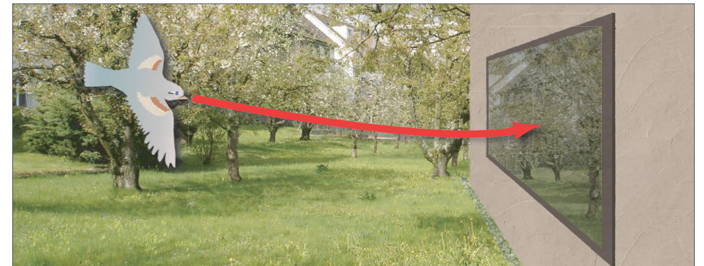
Sun-protection glass and many other types of glass have a high reflectivity index. The stronger the reflection and the more attractive the environment reflected, the greater the number of collisions.
